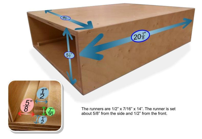
The drawer front fits inside and is flush with the front of the cabinet.
