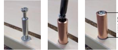
Head of Pin flush with top of Gauge 26 mm
